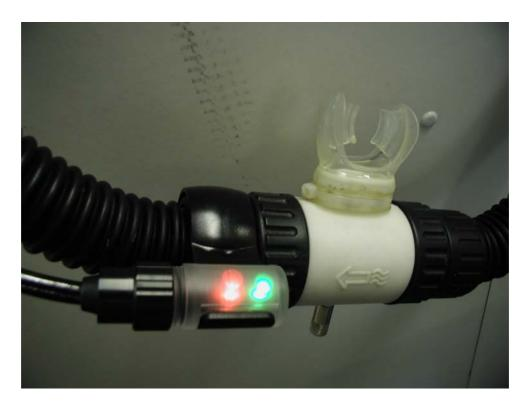
• The Heads Up Display (HUD) is designed to fit on a mounting bracket and attach to the side of the mouthpiece of the rebreather; it contains 2 LEDs, one red and one green.
