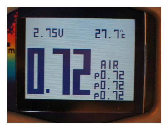
• This is the surface dry screen saver showing battery voltage and temperature along the top of the screen, average PO2 in large numbers on the left, selected diluent on the right and the actual PO2 of the three cells below.
