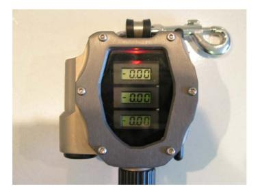
There is a red indicator LED light at the top of the display. When the battery needs to be changed, the red LED will stay on permanently **WHEN A BUTTON IS PRESSED**.
