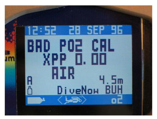
• If the unit is incorrectly calibrated you get the message **Bad PO2 Cal** in the home screen, **do not dive**, check the sensor connections and the health of the cells on the rebreather and repeat the calibration process again.
